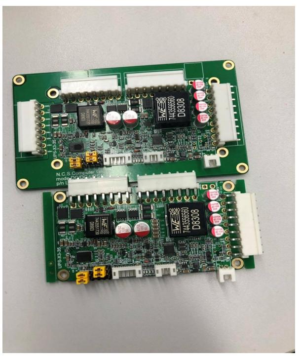
Vout +12 Vdc o +24Vdc /15A - Operating Temperature -40°C to + 85°C dimensions board : 120 (4,72") x 70mm (2,755")
